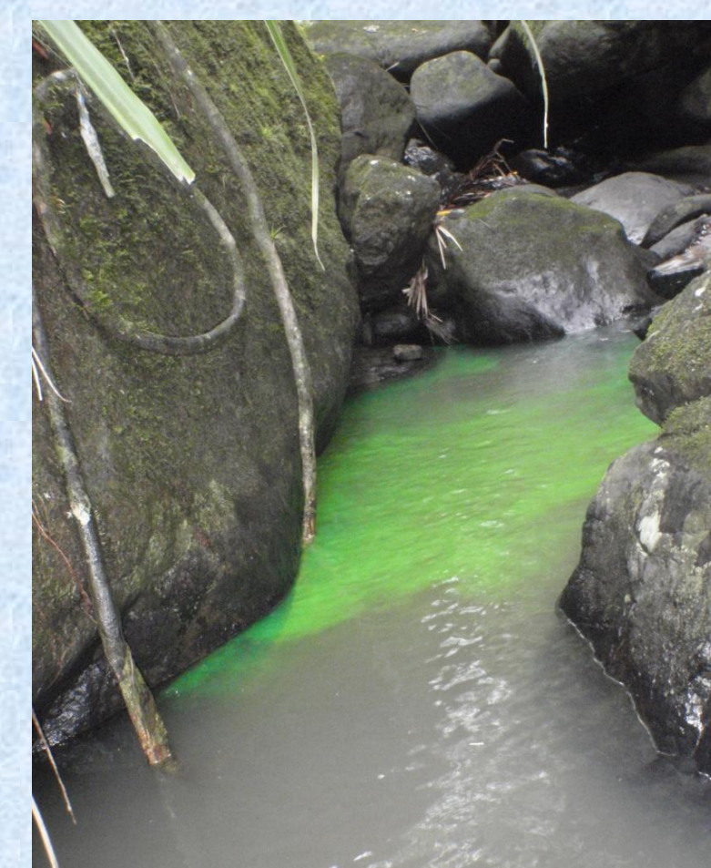
Dye released to measure pool flow.
