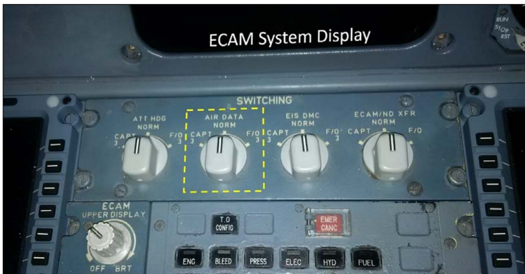
Figure 14: EFIS switching panel. Air data source switch highlighted by yellow box
